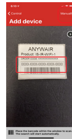
STEP 5 If scanning the barcode, please ensure to use the barcode on the sticker, not on the unit. Alternatively, you can add the registration number by clicking "Manually".
