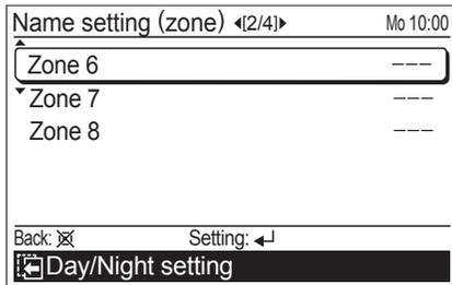
2. Select the zone to be named with the [Cursor button (Up/Down)], and press the [Enter button].
