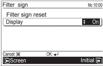
When you set this setting to [On], and air filter cleaning on the indoor unit is required, the icon is displayed on the "Monitor" screen.
