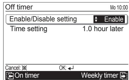
4 For [Time setting], adjust the time with the [Cursor button (Up/Down)], and press the [Enter button] to complete the setting.
