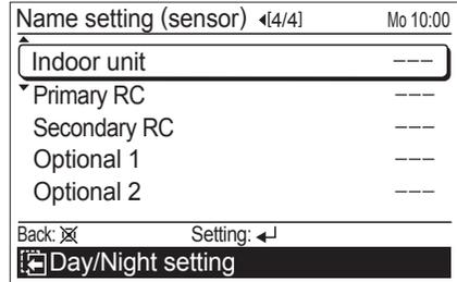
If any names have been registered for the sensors already, the registered names are displayed instead of "----" on this screen.
